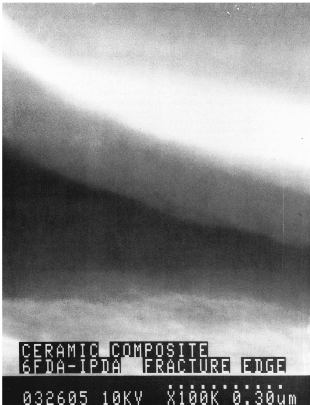
Figure 3 Magnified view of the scanning electron micrograph of the cross section of the composite membrane shown in Figure 2. Photograph taken at a magnification of 100,000 \times and 10 kV.
